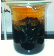
Composite Specimen in Nitric Acid
